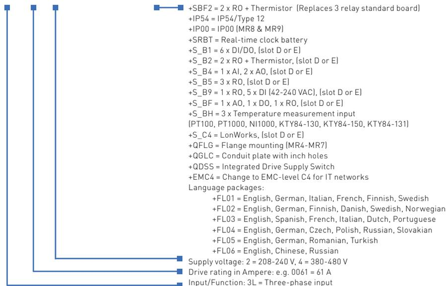
Standard delivery includes IP21/ Type 1, EMC level C2, graphical display keypad, relay board 1 +SBF1 (3 x RO) and +FL01.
